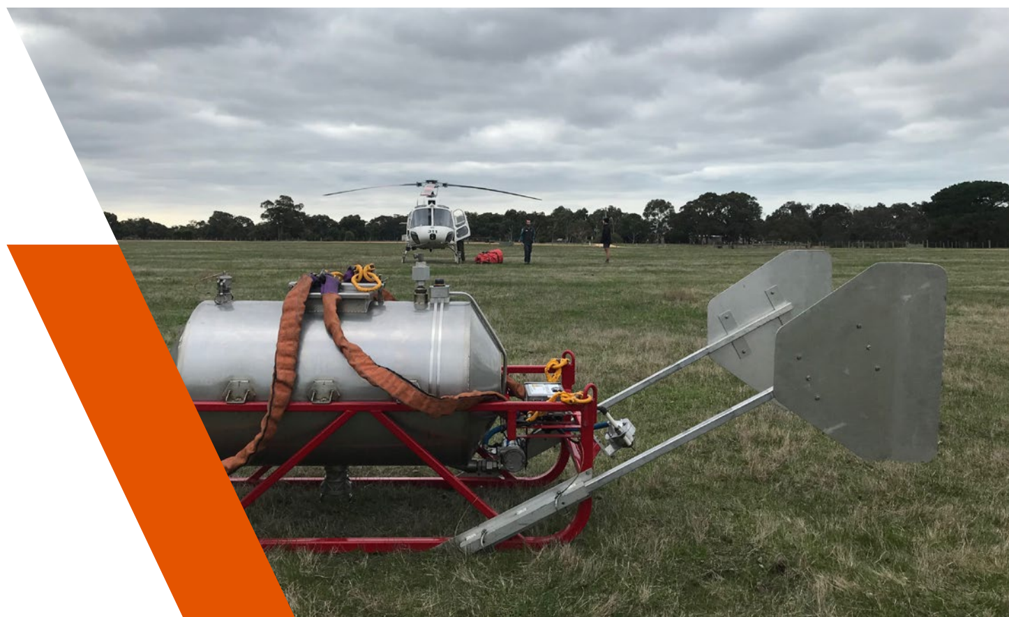
Image 4. Aerial driptorch, an increasingly important tool to achieve fine-scale mosaic outcomes across target parts of the landscape
