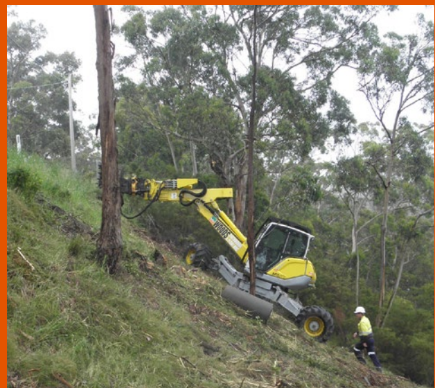
Image 6. Outcomes of Mulching treatments (Left) and mulching on steep slopes being undertaken using an all terrain or 'spider' excavator (Right). Mechanical fuel treatments, like mulching, assist in the safer delivery of planned burns by treating part of a burn unit which has complex vegetation or topography. This type of fuel treatment is also very effective where planned burning is not operationally feasible due to dispersed houses and other assets in a forested area. Mechanical fuel treatments are not weather dependent like planned burning, enabling us to reduce fuel loads in priority locations every year. These works will target the understorey vegetation leaving the larger remnant trees in place.
